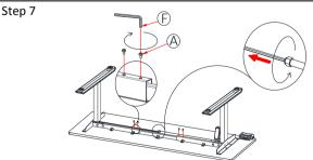
Tighten Crossbeams (part 6) using (part A) Screw M6x10. Adjust the Hexagonal rod (part 7) to the proper position and tighten the plastic
