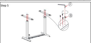
Attach Foot (part 1) to the Lifting leg (parts 2 and 3) using (part B) Screw M6x16.
