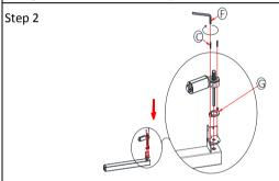
Insert the Hexagonal rod assembled in Step 1 into the hexagonal hole of the Right lifting leg (part 2) through the Motor Gasket (part G), and tighten it with (part C) Screw M5x30.
